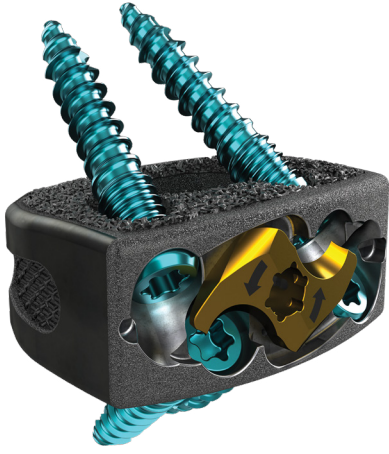
Figure 10: Harrier® SA Standalone ALIF System has an integrated cam-locking mechanism and a large graft window for use with biologics. The interbody cage has three lordotic options of 10, 15, and 20 degrees in three footprints: 26 x 32mm, 28 x 36mm, 30 x 40mm. The implant heights are 12, 13.5, 15, 17, 19mm.
