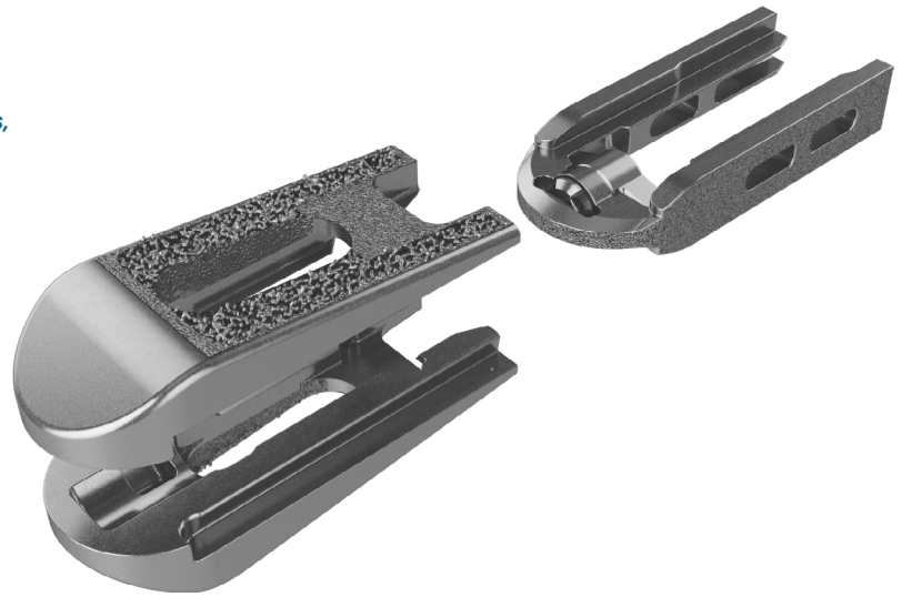
Figure 8: TigerShark® M is a 3D Printed Titanium Lumbar Interbody with a modular in-situ design to minimize the insertion profile while achieving impressive height restoration. Available at a 10mm width with either 6° or 12° lordotic endplates, 2-8mm spacer options in 1mm increments.
