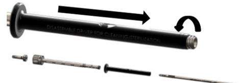
3. To reassemble after cleaning, first thread the sleeve back onto the main driver assembly, then reverse Steps 1 and 2 for driver disassembly by inserting the inner shaft back into the main driver assembly from the bottom. Press the quarter-square connection back onto the inner shaft. An audible/tactile click should be heard/felt. Test the assembly by pushing and pulling on the inner shaft while holding the quarter-square connection fixed. Thread the sleeve back onto the driver assembly.
